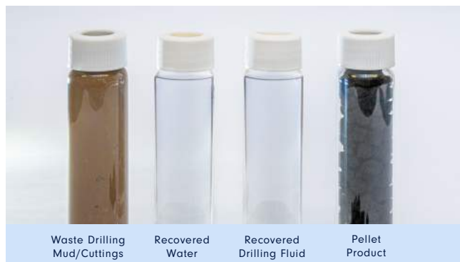
Figure 2: Raw Feed and Outputs from the Vacuum Assisted Pure Oil Recovery Technology
