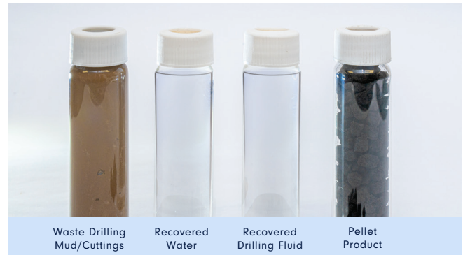
Figure 2: Raw Feed and Outputs from the Vacuum Assisted Pure Oil Recovery Technology
